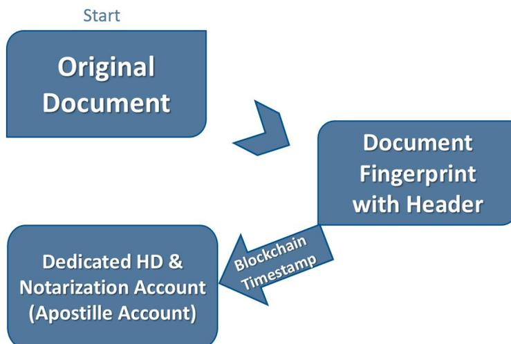
*Figure 6. The Apostille process for creating an Apostille transaction message. The document's fingerprint plus Apostille header are sent in a message to a dedicated HD account.*
